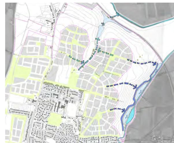
4. Surface water runoff - connections
